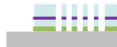
3. ICP plasma etch in Cl<sub>2</sub>/N<sub>2</sub>
