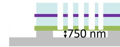
4. Membrane release in XeF<sub>2</sub> vapor
